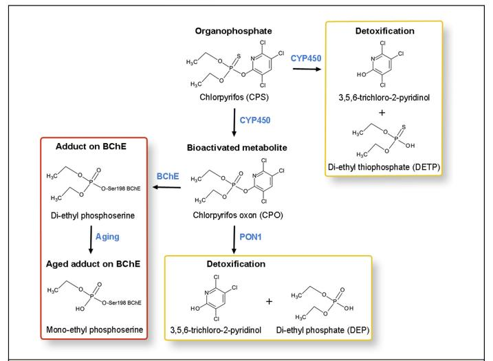
Figure 4. Biotransformation of the organophosphate insecticide chlorpyrifos. The chemical structures in yellow boxes are dialkylphosphate metabolites. The red box contains organophosphate-adducted BChE. BChE, butyrylcholinesterase; CYP, cytochrome.
